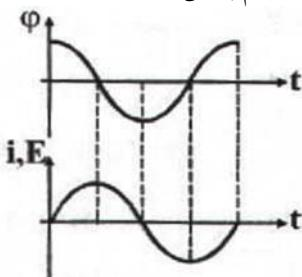
$$\varphi = BA \cos(\omega t) \Rightarrow \varphi = \varphi_m \cos \omega t \quad \omega = \frac{2\pi}{T} = 2\pi v$$
